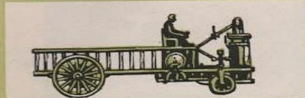
1827 Steam wagon of Onesiphore Pecqueur, France, allowed for difference in rear wheel speeds.
