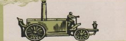
1832 Steam vehicle by W. H. James, England. It had the first three-speed transmission.
