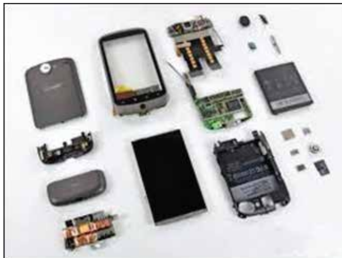
Fig: 2.4.2.3 Mobile Phone Hardware
