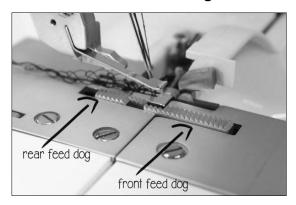
Feed dogs feed from below only. While sewing through two layers of fabric, it is quite possible that both layers get fed at different rates.
