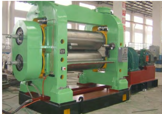
Fig. 1.2.7. 2 roll calender vertical type
