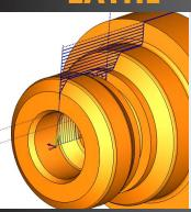
Lathe CAD-CAM makes it easy to set facing and OD/ID roughing, finishing, threading, and grooving 2 axis toolpaths on your CNC turning machine. Define custom tool holders, inserts and part holders for a realistic simulation experience to give you the peace of mind in knowing what will occur at your actual machine before ever cutting a chip.
