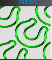
Powerful true shape nesting algorithms provide faster and smarter sheet optimizing functionality to increase your per job profitability with higher sheet yields on your nesting jobs. Batch processing allows you to upload multiple part files to a single nesting job while part-in-part nesting lets smaller parts be positioned inside of larger parts to maximize overall sheet usage. This is an advanced shape cutting solution designed for CNC mill, router, laser, plasma, and waterjet shops.
