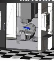
Visualize your machine in action within the CAM simulation window to test and confirm your toolpath programming on 2-5 axis CNC machines. This allows you to verify part fixtures are oriented correctly, machine movements are collision free, proper tool fixtures sizes are being used, and much more. The simulation play controls and move list allow you to easily isolate potential programming problems and quickly make the required adjustments.
