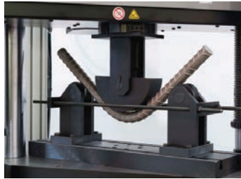
Fig. 1.2.12 Reinforcement bars during bending
