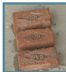
Brick absorbs < 5% of its weight - Good quality
