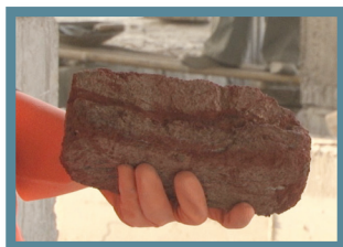
Brick with impression - Poor quality
