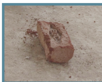
Brick breaks when dropped - Poor quality
