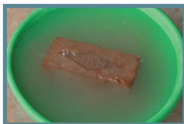
Brick absorbs < 5% of its weight - Good quality
