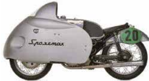
Fig: 1.4.1.5 NSU Sport max streamlined motorcycle, 250 cc class winner of the 1955 Grand Prix season
