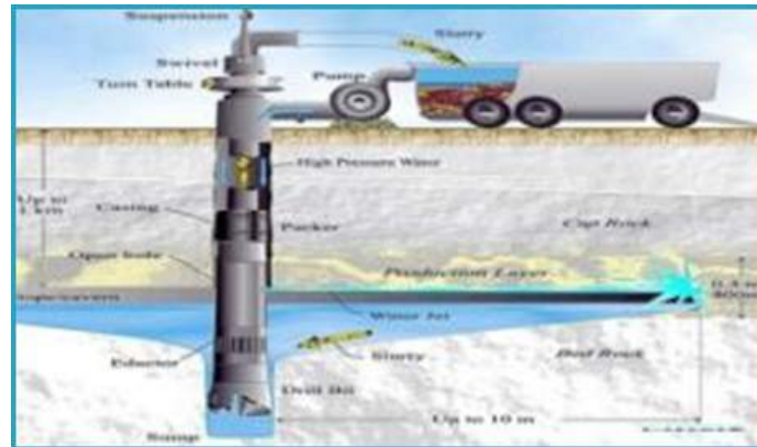
Figure 1.6 : Borehole mining
