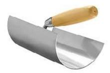
**Step trowel:** Is a type of trowel used for shaping inside angles on concrete steps. The center of the 90-degree bend in the blade allows for rounded edges
