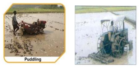
(a) Using power tiller (b) Using tractor-operated puddler
