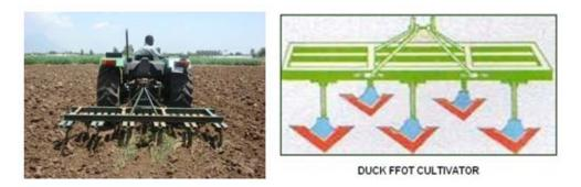
Fig. 1.19 : Different types of tractor drawn cultivators
