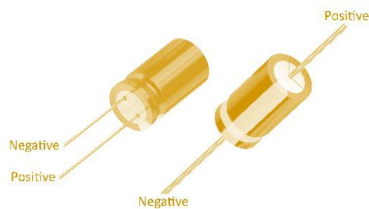
Fig. 1.1.18: Polarity in electronic components
