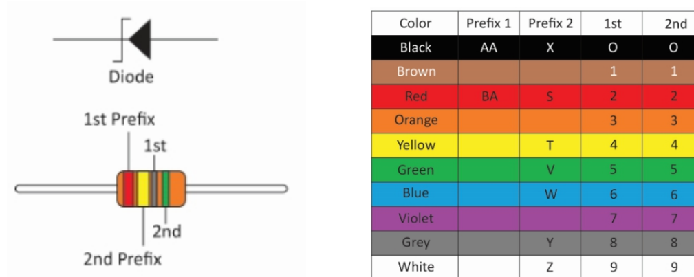
Fig. 1.1.16: Colour coding in diodes
