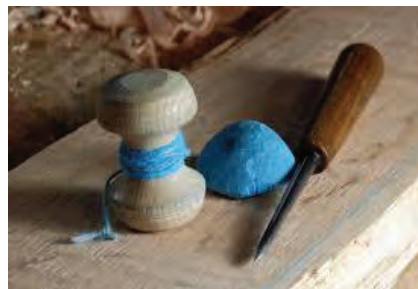
Fig. 1.3.9.7: Marking Thread or Chalk line
