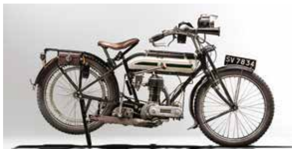
Fig: 1.4.1.4 Triumph Motorcycles Model H, mass-produced for the war effort and notable for its reliability
