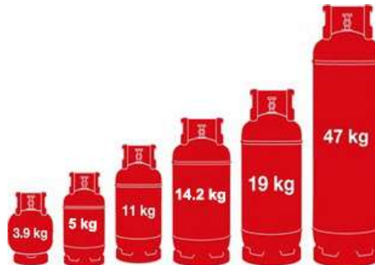
Fig. 2.1.7. LPG cylinders sizes and capacities
