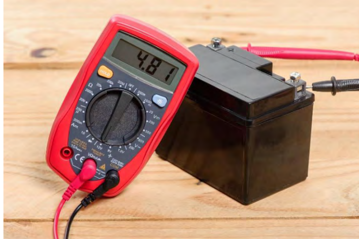
Fig. 1.1.5: Measurement of DC voltage
